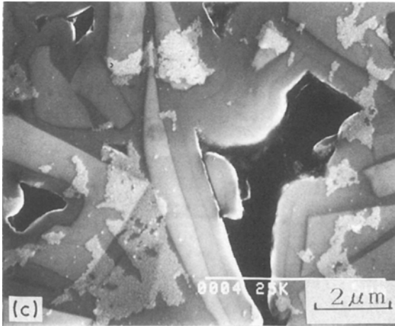
Figure 10 Cross-sections at various depths after 30 000 pulses of CVI into 4 \mu\text{m} particulate substrate at 1273 K. Depths ( \mu\text{m} ): (a) 100, (b) 300, (c) 500.
